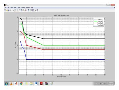
When the overcurrent curves are applied to a piece of equipment and the energy through the equipment is calculated, it can be seen that the energy increases exponentially. Figure 4.10 depicts energy through a 6 inch piece of copper over a range of currents. In the equation for energy, the resistance is held constant; independent of the current. As the current increases the total time the current is applied to the equipment decreases due to the inverse overcurrent curve. Since the
