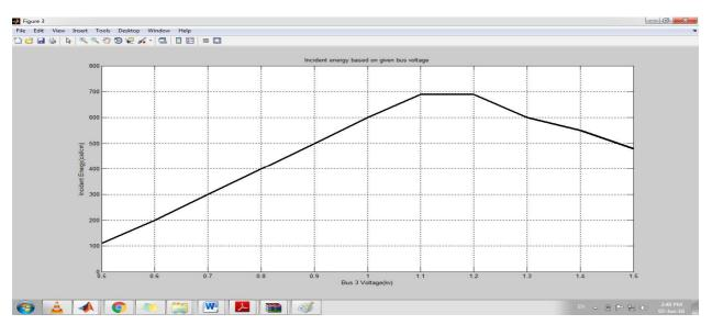
The opposite trend is found when only using the equation for equipment above 1 kV and less than 15 kV. As it shows, the incident energy increases as the voltage increases until it reaches 1 kV. At this point, the equation for equipment above 1 kV and less than 15 kV takes over and we see a slight increase in incident energy up to 1.1 kV and then the incident energy decreases. The discontinuity can be associated to two factors. First, in the equation for equipment less
