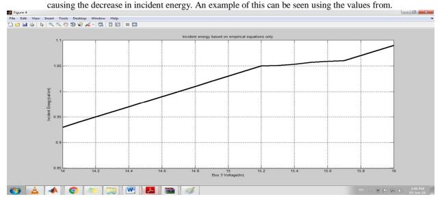
the test system. When the voltage is at 900 volts, the lgIa is equal to 3.55 kA when using equation (3.1) and 3.76 kA when using equation (3.2). When the voltage is at 1.1 kV, the lgIa is equal to 3.92 kA when using equation (3.1) and 3.68 kA when using equation (3.2). If the voltage was to be applied in the equation (3.1), there would be a multiplying
