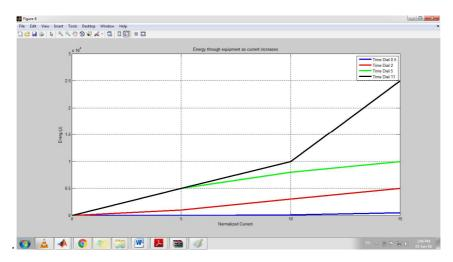
Now looking at the plots of the incident energy in Figure 4.11, using the same overcurrent curves and range of currents, the incident energy is linear. This is due to the fact that never in the equation is the current squared.
